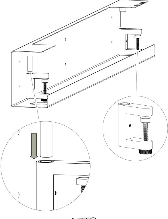
When the multi clamps have been connected to the tube, then open the finger screw entirely before continuing.
