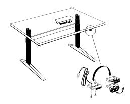
The DPA can be mounted on the desktop so that the keys are either facing upwards or outwards.
