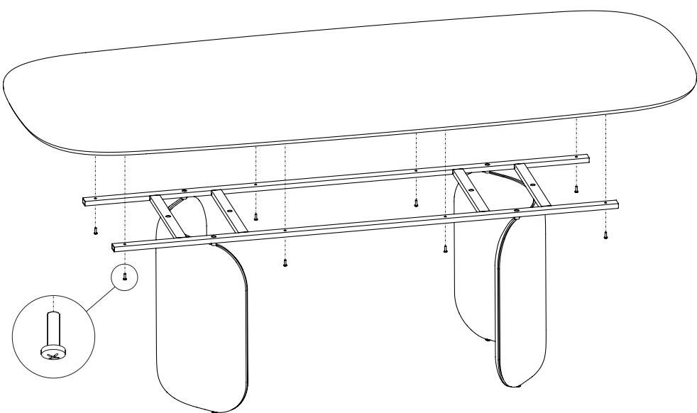
**EN** - 3) Fix the top on the metal frame using the supplied screws. If necessary, adjust the feet to stabilise the table.
