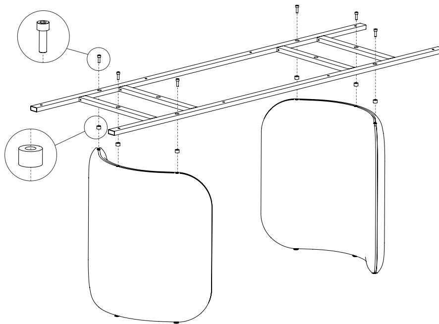
**EN** - 2) Insert the spacers between the bases and the metal frame fixing them with the supplied screws. For the rectangular versions of the table, it is possible to position the bases as shown in the above image.
